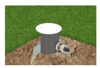
The underground socket is closed with the enclosed wrench and the space around the base box is filled with mortar and filled with soil, grass, etc. The drawer lid must be tightened firmly / well with a wrench to ensure that the socket is covered.
