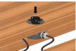
The socket holder, including the sockets themselves, is removed from the box and the cable (s) are passed through the bushing into the box and the bushing is tightened to the cable. The cable (s) are connected to the appropriate socket and the socket holder is attached back to the floor box. The cable entries (instead of the cable entering the bushing) must be secured (eg with a sealing compound) so that the supply is sealed and water / moisture does not get into the socket.
