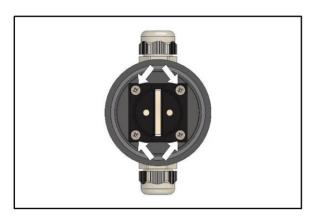
First, unscrew the lid and possibly the bushings (if they are already prepared in the base box). Furthermore, the socket holder, including the sockets themselves, is removed from the box. Note: the 230V socket is always delivered according to the standards on the relevant market. For the Czech Republic and Slovakia with a safety pin.
